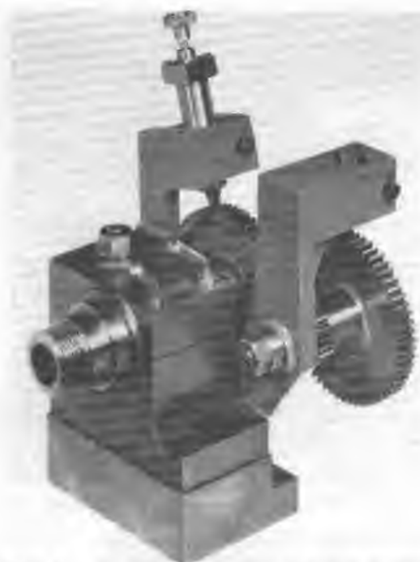
Fig. 53 The M.E.S. Direct Division Dividing Head. This is only supplied as a kit of parts suitable for home construction.
